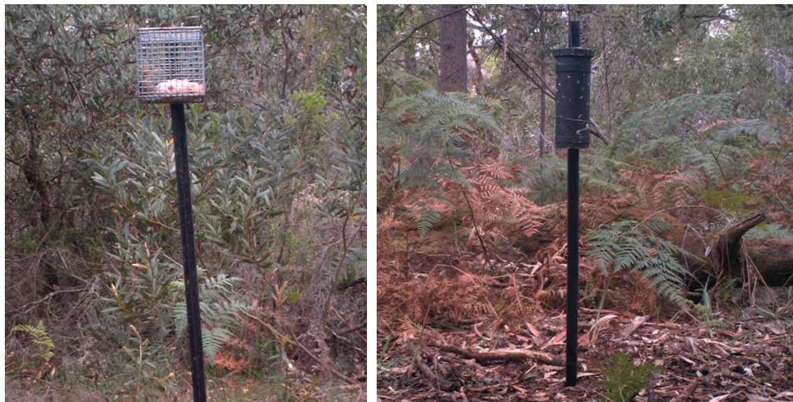
Figure 4. Bait holders used in this study: (a) small wire cage, (b) PVC tube.
