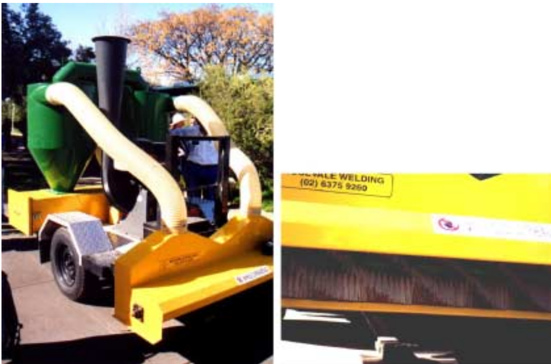
Figure 5 'Rosevale Reaper', a combined brush and vacuum harvester.
