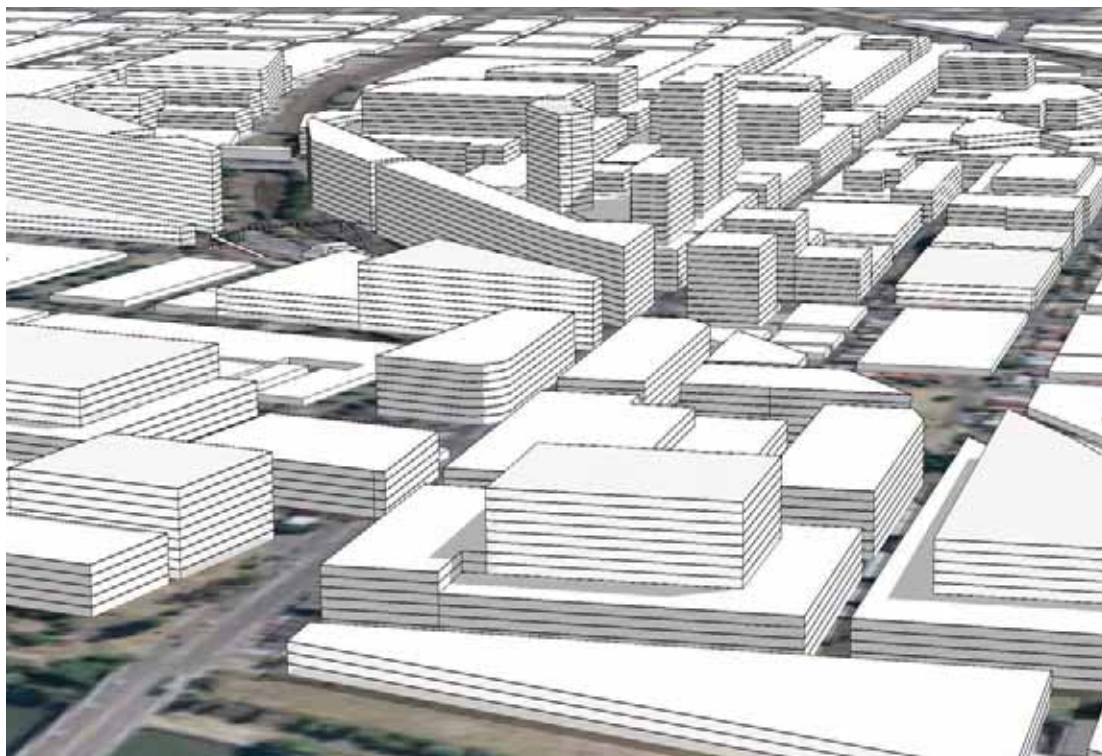
Figure 3 – Urban Massing Study - Scenario 2 Heights of 20-25 storeys on Market site and 15 storeys on triangle site. (Source SJB Urban)
