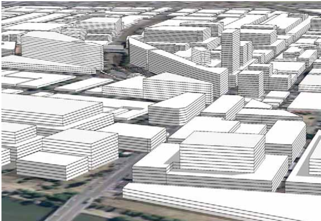
Figure 2 – Urban Massing Study Scenario 1 – Height of 12-15 storeys on Market site and 20 storeys on triangle site (Source SJB Urban)
